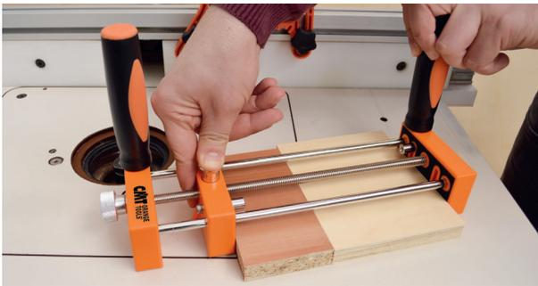
**2.** Press the Quick Release Button [E]. Slide the Adjustable Center Base over until it rests snugly up against the small stock piece you are working on. Ensure that your small stock piece is always lying flat on the work table surface. Release the Quick Release Button. In the image, a "sacrificial" piece is being used in order to prevent tear-out.
