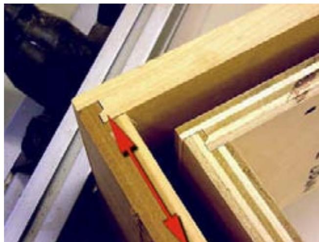
Before we leave this bit, here is an easy way to add a specific amount of overlap. First, set the fence using the set-up blocks to have a "flush" fit. With your test piece against the cutter and your ruler at the center point of the bit, move the fence back to give you the distance equal to the rabbet you want.
