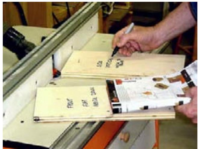
It doesn't matter which component is cut first. I opt to run the front/back piece first. The pushpad keeps the board flat to the table and gives me positive and safe control.
