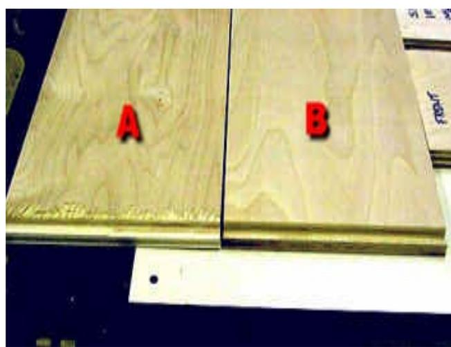
That's right. In the initial setup, I simply moved the split fences to be close to the left and right sides of the bit. The tearout is not at the ends but above the cutter. Since the CMT Router Table allows the use of inserts, making the customized insert was as simple as could be – and made all the difference in the world.
