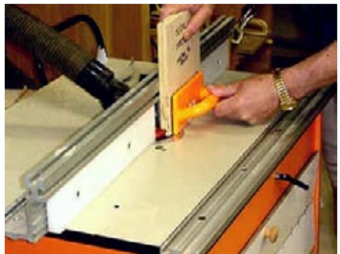
Several test cuts later, and I have learned quite a bit about setting up this bit. First, I make no adjustment to the height of the bit. The initial 15/64" is ideal for 3/4" stock.
