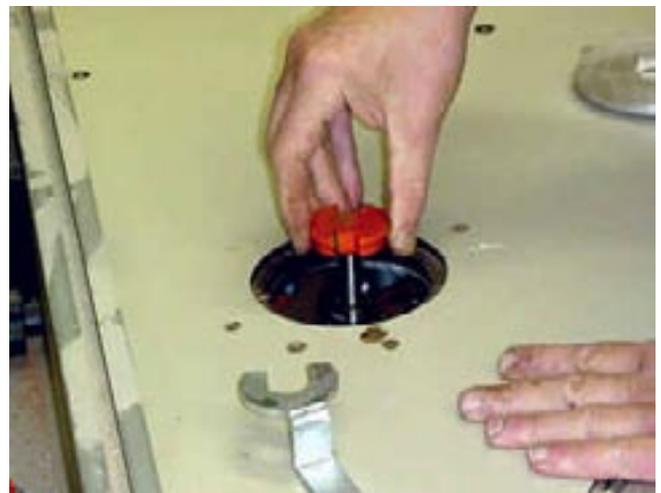
I unlock the router plunge mechanism and adjust the bit height so that the middle of the bevel is 15/64" above the table.
